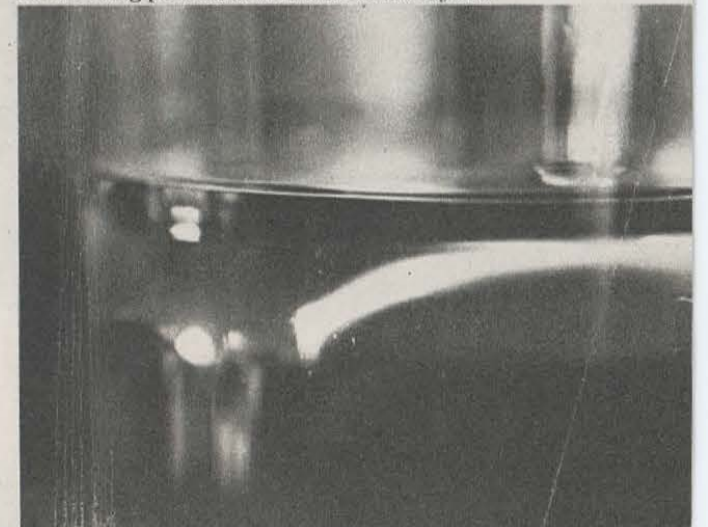
A light shining through the liquids bends at the meeting point. Same is true in air layers.
